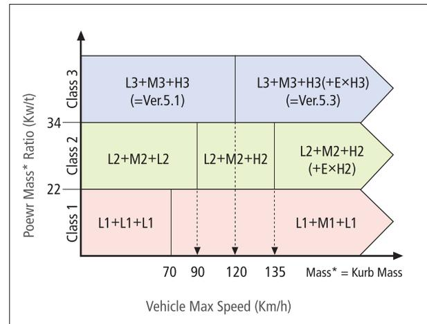
Fig. 4. WLTP driving cycle allocation (Tutuianu et al. 2013)
